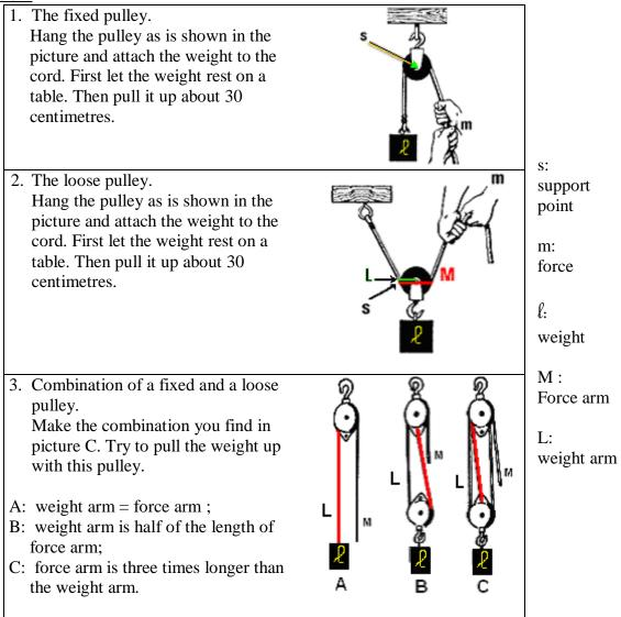
It is easier to lift the weight with the loose pulley than with the fixed pulley. Even more easy is using the combination, but it takes more time.
