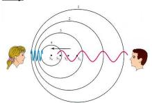
The buzzer has a monotonous pitch, but when it comes closer to the ear, the frequency of the arriving vibration increases, causing a higher pitch.
